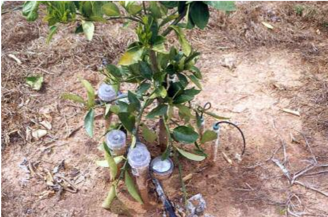
Fig.1. Installed tensiometer in sweet orange
